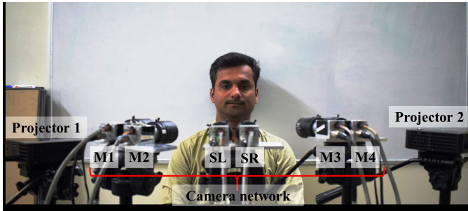
Fig. 5: An instance of the facial surface imaging platform used in this paper. ‘SL’ and ‘SR’ cameras form a stereo pair. ‘Mi’ indicates i^{\text{th}} monocular camera.
